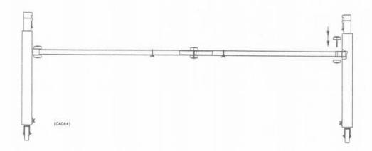
**d.** Assemble (2) diagonal crossbar braces (to the crossbar and end pieces) with wing nuts as shown.
